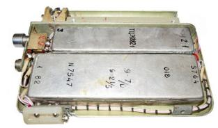
'Cigar case' radio with top cover detached showing 2 sealed modules and the battery compartment.
